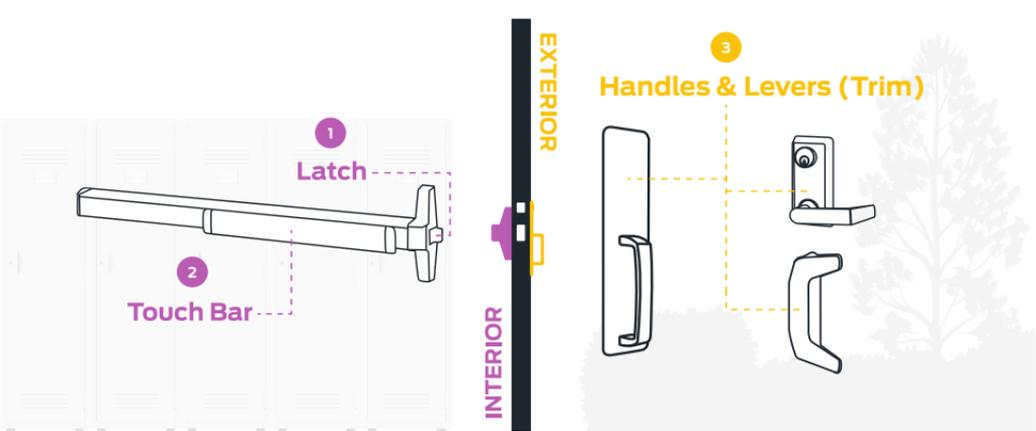
★ When a panic device's touch bar is pushed in, this pulls back the latch bolt so the door can be opened.
