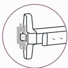
The device's latch bolt is engaged with the strike on the frame, or in the floor and frame if the device has latch bolts at the top or bottom of the door.
