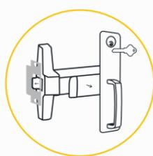
Only a key or credential can unlock the outside. For a panic device to be locked, it must also be latched.
