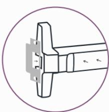
A device is dogged when the latch bolt of the panic device is held retracted so that the door can be easily pulled open from the outside trim. The door must be undogged to be secure.
