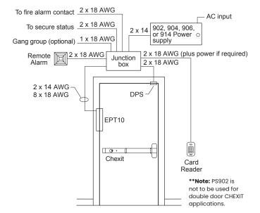
Figure 1. Riser Diagram, Single Door
